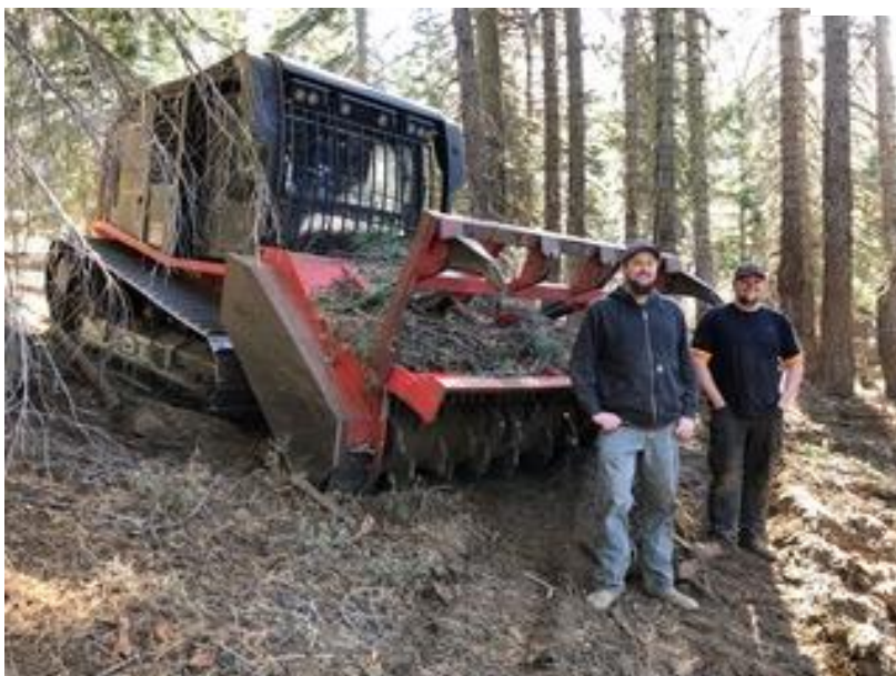
Local Tree Thinning Crew: Local contractors from Camp Connell stand next to a large masticator they are using to selectively thin the forest to reduce the risk of catastrophic wildfire and improve the health of the Mokelumne watershed.
